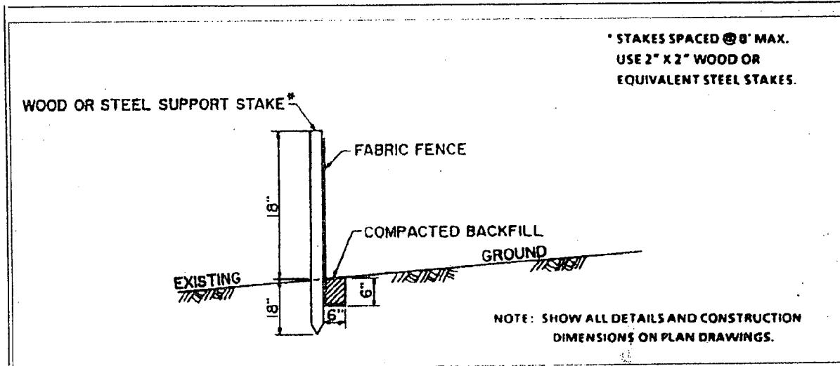
Filter fabric fence must be installed at level grade. Both ends of each fence section must be extended at least 8 feet upslope at 45 degrees to the main fence alignment.
