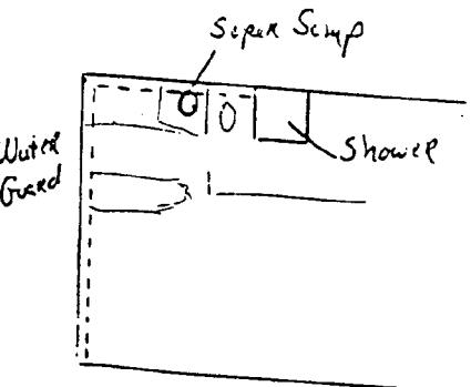
Note: Owner will have cubboards, heating units, and any other items against the wall removed before our arrival. We will remove approx 2 ft of the drywall, cut off the studs, and pin it to the wall, to support the wall.
