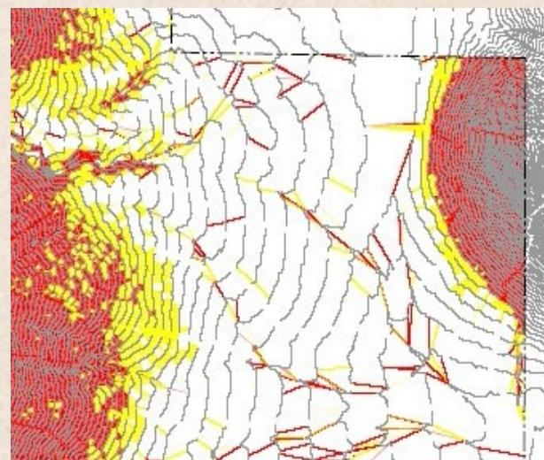
A slope gradient study maps the steepness of natural slopes to assist in evaluating the appropriateness of grading. Steeper areas are signified by red and yellow colors.
